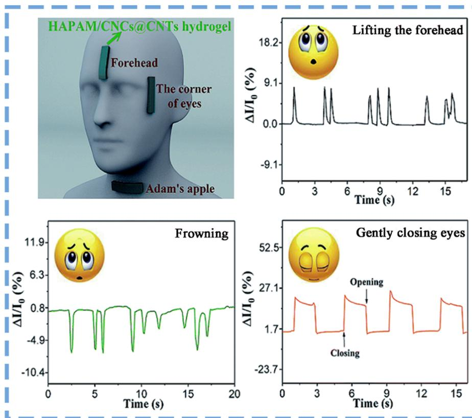
Fig. 16. CHs-based highly sensitive strain sensor attached to the forehead, the corner of the eye to detect facial expressions and corresponding current responses. Reproduced and reprinted with permission. Reproduced from ref. [395] with permission from The Royal Society of Chemistry, copyright 2019.
