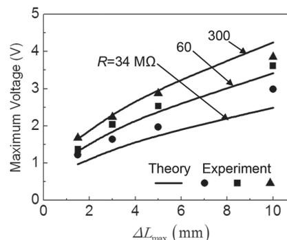
**Figure 4.** Comparison of the maximum output voltage between theory and experiments for the resistance of 34, 60, and 300 M $\Omega$ .
