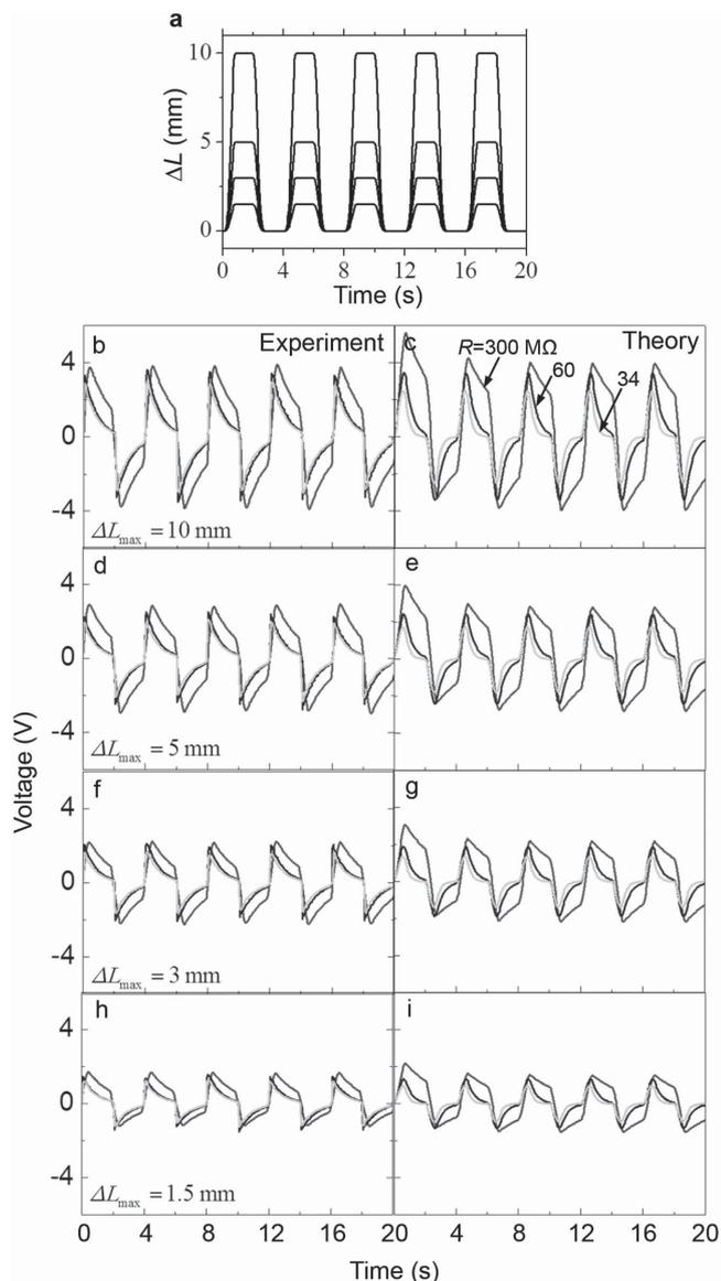
**Figure 3.** a) Displacement load and the comparison of voltage between b,d,f,h) experiments and c,e,g,i) theory as functions of time for resistance of 34, 60, and 300 M $\Omega$  and maximum displacement of 1.5, 3, 5, and 10 mm.
