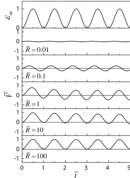
**Figure 6.** Effects of the dimensionless resistance on the dimensionless voltage.
