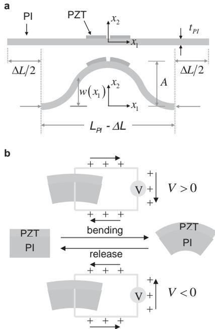
**Figure 5.** Schematic illustrations of a) theoretical shape for buckling of a PZT MEH under compression and b) charge movement in the circuit during the cycling load.
