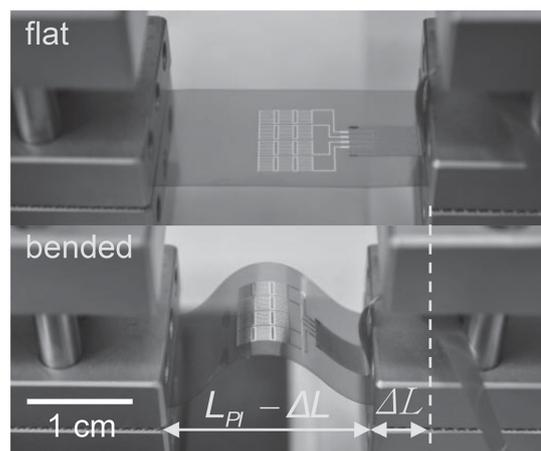
**Figure 2.** Photographs of a PZT MEH clamped on a bending stage in flat (upper) and bent (lower) configurations.
