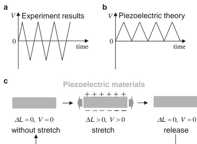
**Figure 1.** Schematic illustrations of the curves of output voltage versus time from a) experiments and b) piezoelectric theory for open circuit. c) Schematic illustration of the voltage and charge distribution of piezoelectric materials subject to stretching.
